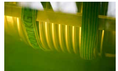
Pressure and leakproof testing in special liquid bath
