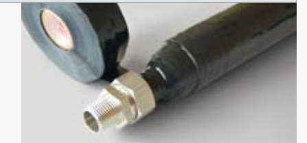
Generously apply silicone adhesive to the end of the insulation. Wrap silicone self-adhesive tape with a 50% overlap around the end up to the screw coupling.
