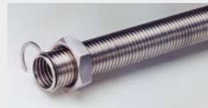
Fit clamp ring into first corrugation groove and compress it to form a closed ring. Insert gasket. Place threaded male connector in end of hose and tighten with two open-end spanners.
