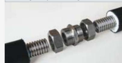
Remove approx. 6 cm of the insulation. Fit the connection fitting. Generously apply silicone adhesive to the end of the insulation.
