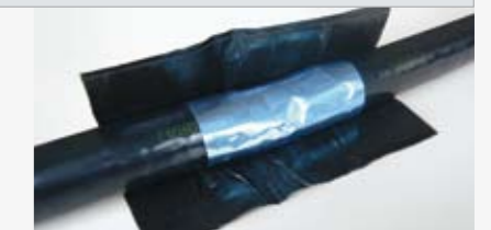
Wrap the rubber mat around the assembly. It should overlap the taped assembly by approx. 2.5 cm on each side.
