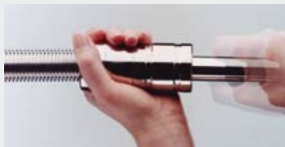
Close clamping jaw and use the striking pin to compress the corrugation into the form of a rim.
