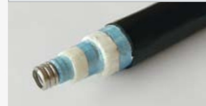
Remove approx. 6 cm of the insulation in three steps
