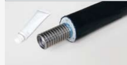
Remove approx. 6 cm of the insulation. Generously apply silicone adhesive to the end of the insulation.
